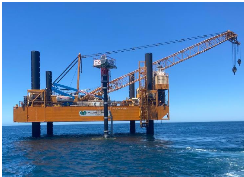
Jack up barge used for construction
